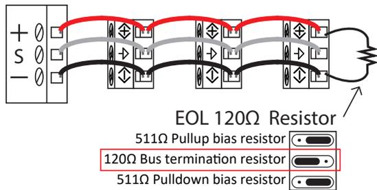
Use of appropriate shielded twisted pair wire (14-26 AWG) is recommended, per protocol specifications. Total wiring runs should not exceed 4000 feet, with a maximum of 128 devices (BACnet) or 32 devices (Modbus) in a single daisy chain.
